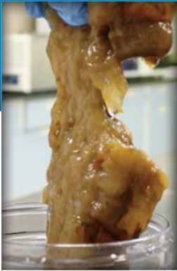
Common sugar snake buildup found in beverage tower drains
